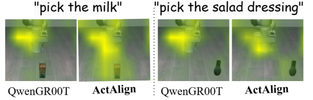
Figure 7: Cross-attention visualization between the VLM and action prediction head. ActAlign focuses more on action-relevant regions (e.g., movable areas and robot end-effector), beyond the target object.
